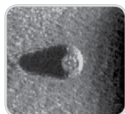
Side scan image of a mine-like object captured at 900 kHz.
