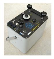
The prototype has a drift rate of approximately 0.030 mGals per month. The Burris Gravity Meter™ has consistently yielded standard deviations of 0.003 mGal or better during routine field tests.
