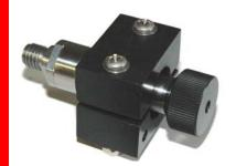
Designed as a scaling device for video and digital cameras, the Ocean Imaging Systems Model 400-37 laser features a titanium housing and connector, sapphire optical port, and an adjustable "ball in socket" mounting clamp. Typically, two lasers (or optionally 4) are mounted and aimed to place two laser "dots" within the field of view of the camera, a known distance apart. The dots serve as a known reference for scaling objects within the image.
