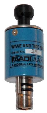
5218/5218R is based on a silicon piezoresistive pressure sensor. The pressure measurements are sampled and temperature compensated by an advanced Digital Signal Processor.
