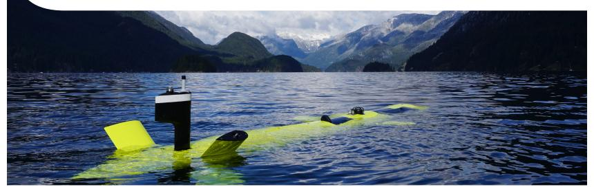
The ISE EXPLORER Autonomous Underwater Vehicle (AUV) collects **IHO compliant data** at a rate of **750 to 1100 km per week** of ship time with all sensors operating and is the most modular and maneuverable AUV in the world today. The modular design of the EXPLORER enables it to carry multiple payloads in its spacious, swappable, and customisable payload section.
