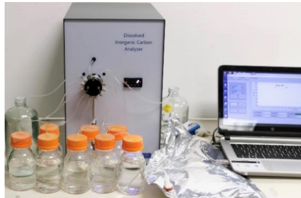
Figure 1. Front view of the DIC analyzer AS-C5 with a multi-port sampler and the LI-850 CO 2 detector (inside the main analyzer)
