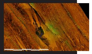
Grid and contour the magnetic field and display it on backscatter imagery.
