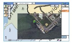
With GPS input, utilizing the range and bearing data, the topside software can calculate and plot the geo position on a chart.
